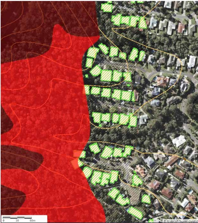
Figure 81: Bushfire Prone Area map 100m potential impact buffer and identified structures. Source: QFES
