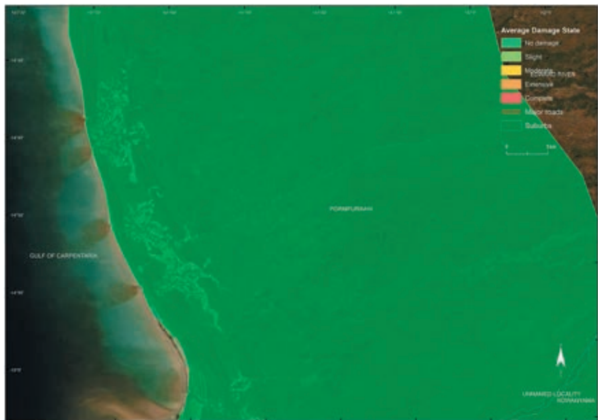
Figure 101: Aggregated residential building damage states for mesh block areas, for scenario 015-09711, a Category 3 cyclone impacting Pormpuraaw, Qld. Note that the spatial aggregation covers very large expanses in this part of Queensland, so any variation in damage within the community may not be discernible on this map.
